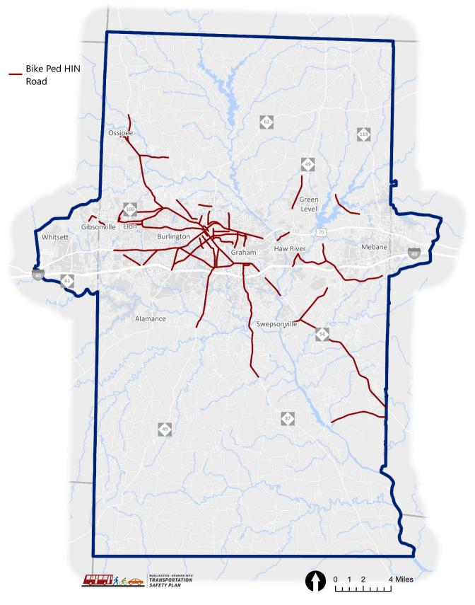
Figure 6.11. High Injury Network – Bicycle, Pedestrian, and Other Nonmotorized Transportation
