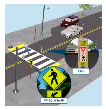
Figure A.5. High Visibility Crosswalk (Source: FHWA)
